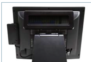
3. VFD customer display unit
